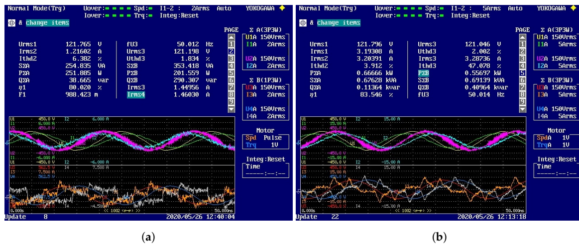
Figure 13. Power analyzers results during asymmetric load-sharing: (a) UPS1 providing 25% of the load power; (b) UPS2 providing 75% of the load power.
