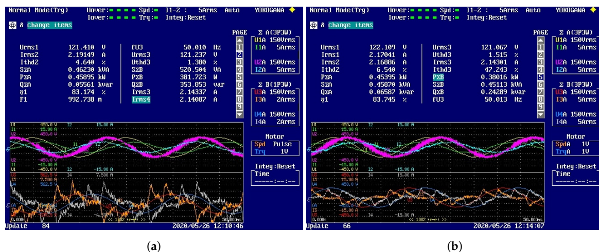
Figure 12. Power analyzer results when the systems are equally sharing the non-linear load: (a) UPS1 providing 50% of the load power; (b) UPS2 providing 50% of the load power.
