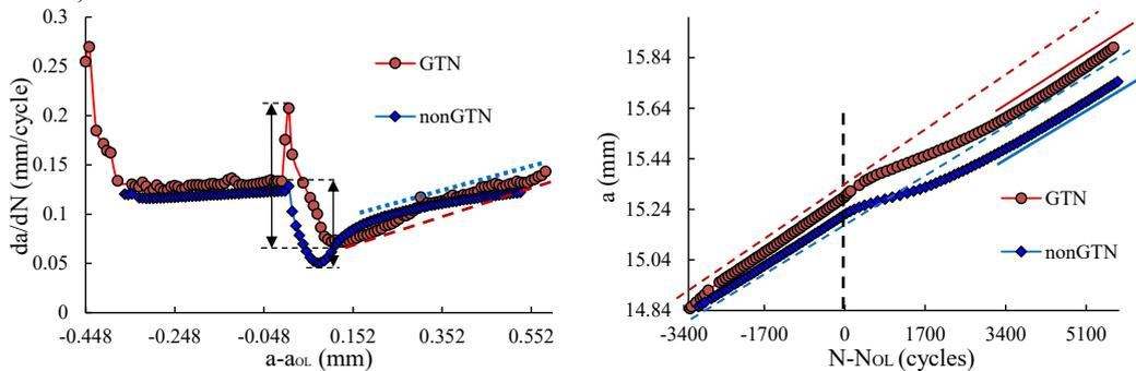
Figure 3. (a)  $da/dN$  in terms of the crack size, in relation to the one verified at the overload application, for both versions of the model. (b) Evolution of the crack size in terms of the applied load cycles, again in relation to the overload application cycle (3300<sup>th</sup>).
