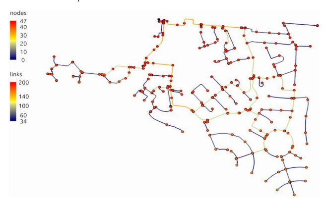
**Figure 3.** Pipe diameters of the infrastructure currently installed. The different colors indicate the diameter for each pipe (links in mm) and the pressure at the nodes (nodes in m) for the deterministic water demand in the hydraulic model (PF = 2.77). The minimum pressure in the network is 34.15 m.
