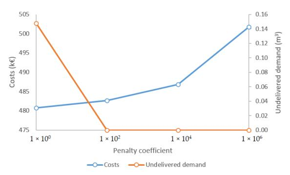
**Figure 8.** Relation between the design costs (axis y1, blue curve) and the total undelivered demand (axis y2, in  $m^3$  during peak hour, orange curve,) for different values of the penalty coefficient (Cpen) in the optimization model when taking future demand scenarios into consideration. Fully satisfying demand under all future scenarios requires higher investment costs in the network.
