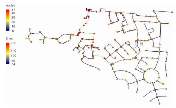
**Figure 4.** Pipe diameters for the optimized deterministic design of the WDN. The different colors indicate the pipe diameter for each pipe (links in mm) and the pressure at the nodes (nodes in m) for the deterministic water demand in the hydraulic model (PF = 2.77). The minimum pressure requirement of 20 m is met at all nodes in the network. Diameters are significantly decreased when compared to the diameters of the currently installed network (Figure 2).
