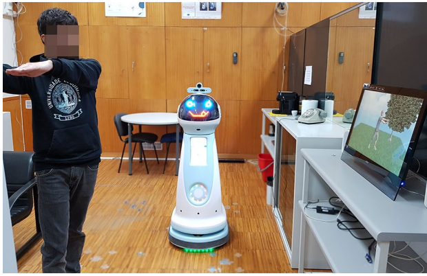
Fig. 3 A user executing exercises accompanied by the robotic buddy and guided by the virtual coach on the screen
