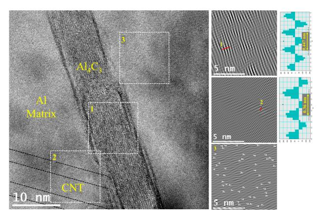
Figure 12. HRTEM image and inverse FFT showing the  $Al_4C_3$ , CNT embedded, and the presence of surrounding dislocations.
