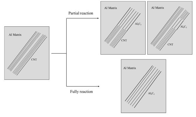
Figure 11. Schematic drawing of different reactions between the CNT and matrix forming the Al<sub>4</sub>C<sub>3</sub> phase.
