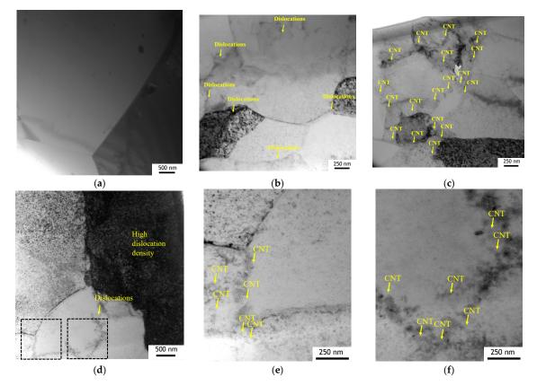
**Figure 9.** TEM images of (**a**) Al, (**b**,**c**) Al-CNTs nanocomposite as produced by ultrasonication sintered during 90 min and (**d**) Al-CNTs heat-treated, and (**e**,**f**) high magnification of regions marked in (**d**).
