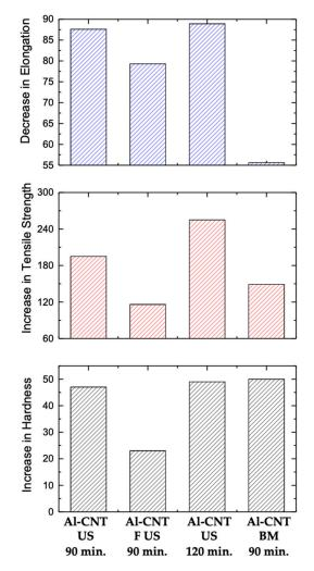
**Figure 4.** Percentage of increase in hardness (HV 0.01) and ultimate tensile strength (MPa) and decrease in elongation (%) for the nanocomposites, concerning the same properties for the Al matrix produced under the same conditions. The designations are the same as in Figure 2.
