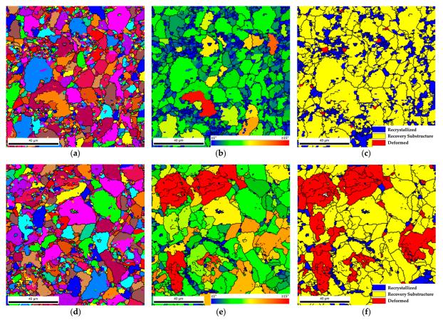
**Figure 7.** Grain size, GOS, and GAM maps of (**a**–**c**) Al and (**d**–**f**) Al-CNTs produced by ultrasonication sintered during 90 min and heat-treated at 480 °C during 90 min.
