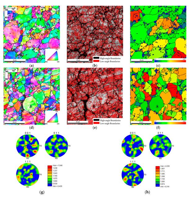
**Figure 6.** IPF maps, IQ maps with high- and low-angle boundaries delineated, GOS maps, and PF of (**a**–**c**,**g**) Al and (**d**–**f**,**h**) Al-CNTs produced by ultrasonication.
