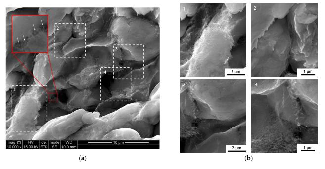
**Figure 5.** SEM images of the fracture surface of nanocomposites produced using ultrasonication: (**a**) lower magnification and (**b**) higher magnification of the regions marked in (**a**) where pulled-out and ruptured CNTs can be observed.
