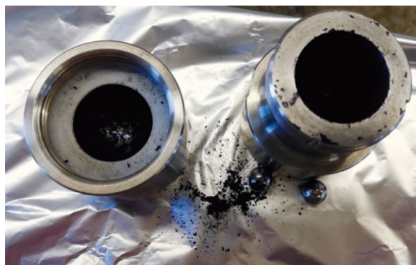
Figure 1. Picture of the reaction crude after 3 h of ball milling.
