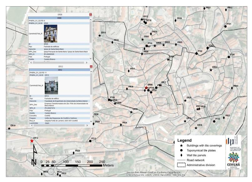
Figure 4. Spatial distribution of glazed tile works considered in a GIS-tool proof of concept developed in partnership with Covilhã Municipality (adapted from [51]).
