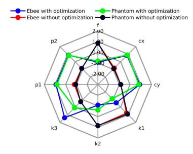
**Figure 10.** Impact of camera optimization step performed in PS-7 on the internal orientation parameters (IOP) for Ebee and Phantom cameras. IOP are f (focal length), principal point (cx, cy), camera position (p1, p2), and distortion parameters (k1, k2, k3).
