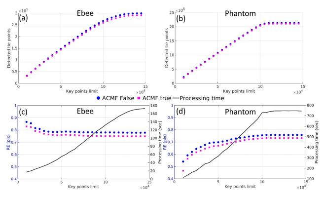
**Figure 5.** Impact of key points limit on the number of detected tie points (**a**,**b**) and on the Reprojection Error (RE) (**c**,**d**) for the Ebee and Phantom image datasets.
