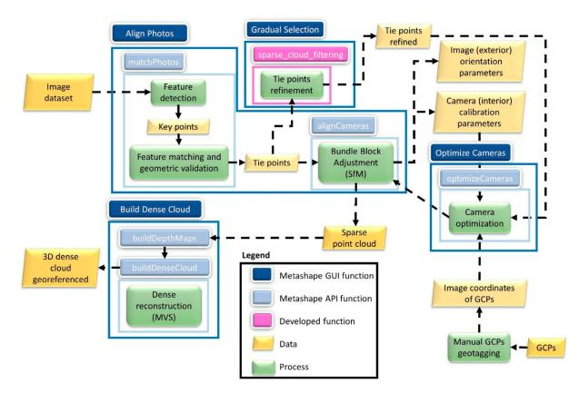
**Figure 3.** The Metashape workflow (blue rectangles) used in the comprehensive analysis superimposed on a typical Structure-from-Motion and Multi View Stereo (SfM-MVS) workflow (green rectangles). The Metashape Graphical User Interface (GUI) functions and their corresponding Metashape Application Program Interface (API) functions.
