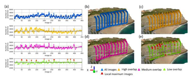
**Figure 11.** Impact of image redundancy (overlap reduction parameter) on the Phantom dataset. (**a**) Impact on the tie point projections. Black lines represent the mean of tie points projections. (**b**–**e**) Impact on the spatial distribution of the images. Colors of graphs lines in (**a**) (blue, golden, magenta, and green) are related to the image acquisition location in (**b**–**e**).
