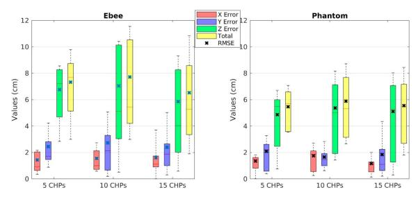
**Figure 7.** Impact of the numbers of GCP on the errors on CHPs for two GCPs distributions for Ebee and Phantom: on the beach and top, using 5 GCPs and 15 CHPs (PS-3) and using 10 GCPs and 10 CHPs (PS-4); on the beach, intermediate level and top, using 15 GCPs and 5 CHPs (PS-5).
