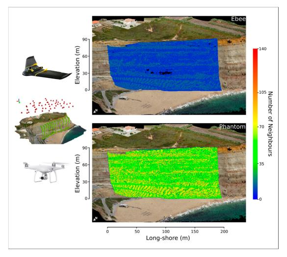
dataset, the superior quality of the characteristics of the dense cloud generated by this dataset is significant. The Phantom (LO) point cloud showed a smaller RE, bigger sparse and dense point clouds with significantly less data gaps.
