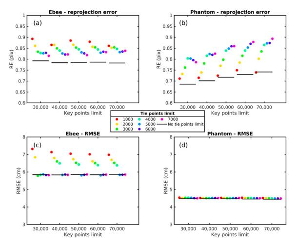
**Figure 6.** Impact of key points and tie points limits on the RE (**a**,**b**) and on the Root Mean Square Error (RMSE) (**c**,**d**) of GCPs, for Ebee (**a**,**c**) and Phantom (**b**,**d**). Colors represent the different values of tie points limit.
