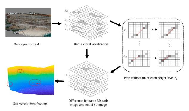
Figure 4. Proposed approach for detecting and quantifying data gaps on 3D dense point clouds.
