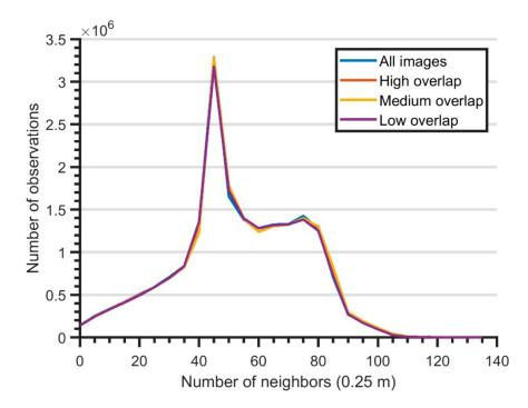
Figure 12. Impact of the Reduce Overlap function on the point cloud density (voxel size of 0.25 m).
