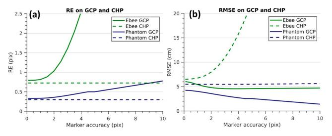
Figure 8. Impact of the observation weights on the RE (a) and RMSE (b) for the Ebee and Phantom image datasets.
