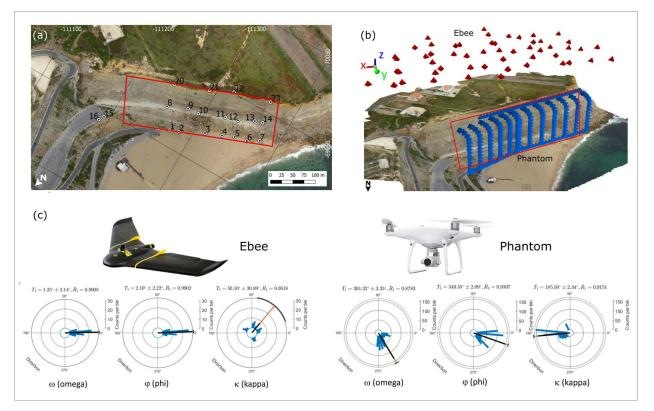
**Figure 2.** Unmanned Aerial Systems (UAS) surveys and ground control point (GCP) location. (**a**) Orthophoto of the study area with the location of the control points (black circles). (**b**) Location of the image centers for the Ebee (red pyramids) and Phantom (blue pyramids). (**c**) Circular distributions of the attitude angles ( $\omega$ ,  $\varphi$ ,  $\kappa$ ) for the Ebee (left) and Phantom (right), with the mean direction ( $\mu$ ) and the resultant vector length (R).
