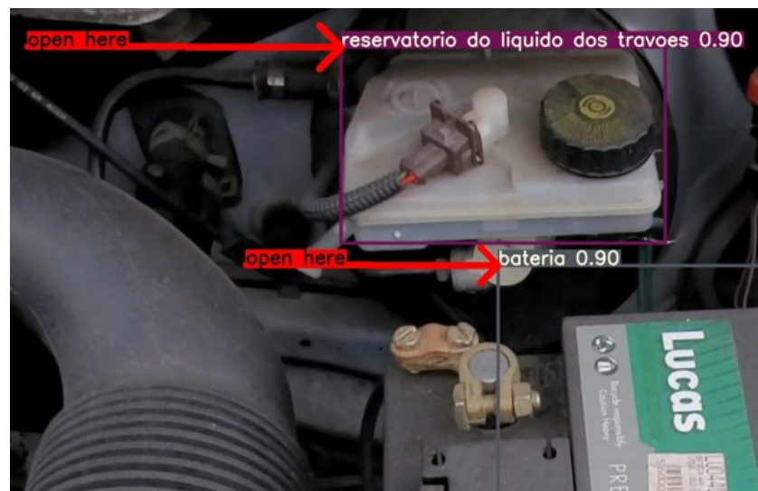
Figure 4. Example of object detection on a test image, where brakes fluid reservoir and battery are detected.
