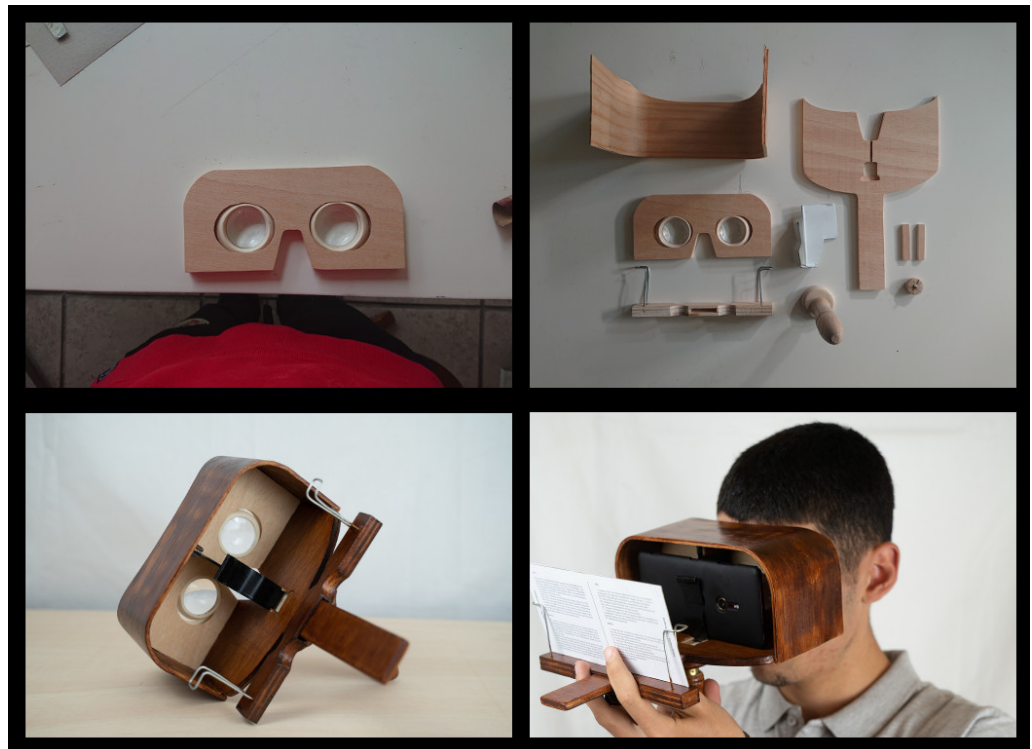
Figure 8. Final device. (Top-Left): Detail of the lenses' mechanism; (Top-Right): Breakout of the components needed to make the device; (Bottom-Left): Device assembled; (Bottom-Right): Usage of the device.
