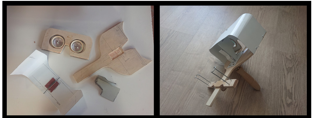
Figure 7. Wood and sheet metal model prototyping process. This model had all the characteristics of the previous paper model, but was made more resistant by the use of materials used in the final stages of prototyping such as wood and metal.
