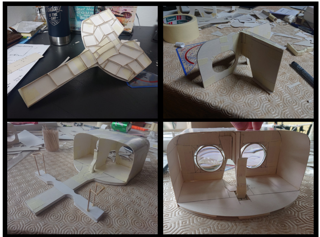
Figure 6. Final paper model prototyping process. It was necessary to understand how several parts would need to be created in more durable materials in the next iteration, such as the card holder and the smartphone support piece. Other parts have been added, such as the part that blocks light from entering the device. The card holder was needed to support the stereoscopic cards that would be read by the software that runs on the smartphone. ( Top-Left ): Detail of the interior of the base showing how we added thickness and rigidity to the paper prototype; ( Top-Right ): Detail of the interior of the head of the device; ( Bottom-Left ): Device with stereocard holder; ( Bottom-Right ): Detail of the movable smartphone support piece.
