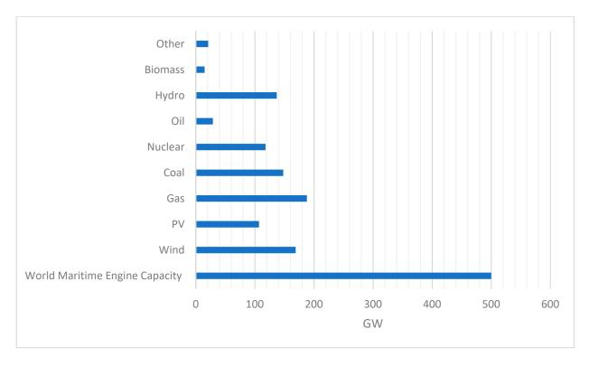
**Figure 1.** World maritime engine power compared to European installed power (The figure was constructed based on data captured from Balcombe et.al (2019) [12] and Statista (2020) [15].
