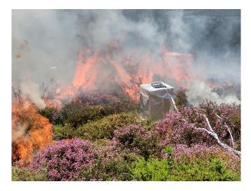
**Figure 2.** Field test (PSS) views during the arrival of the fire front at the protective device of the gas cylinder.
