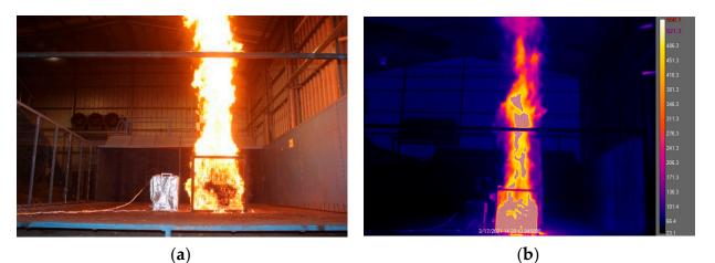
Figure 3. Laboratory test (PS025) at 0.25 m from the basket fuel: (a) video and (b) InfraRed camera image.
