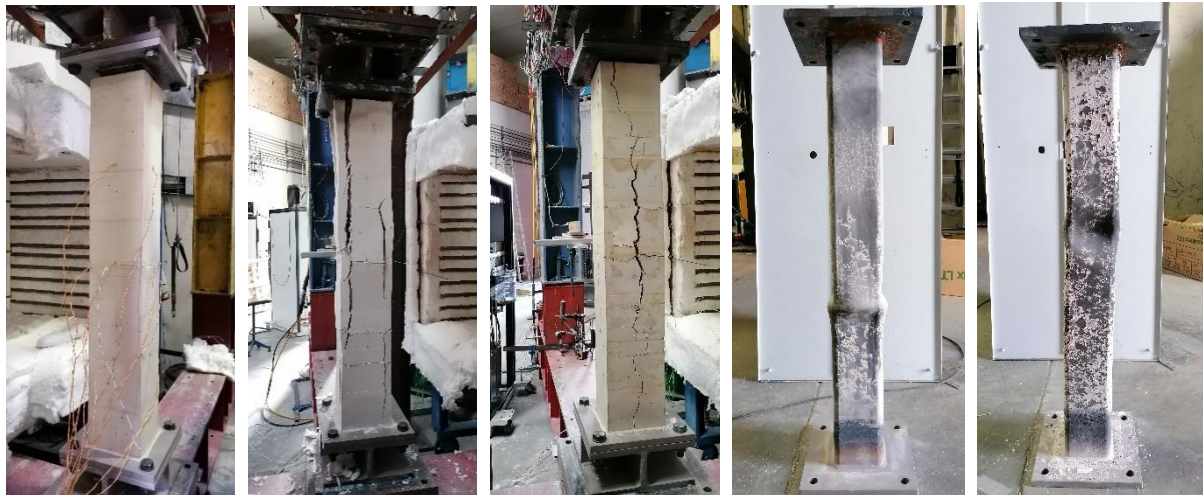
Figure 14. Photos of the specimens of SSC before and after tested, as an example.
