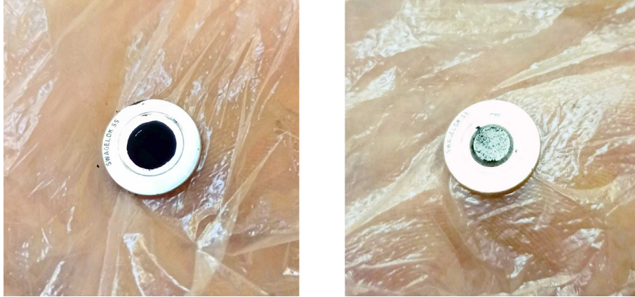
Figure 4.22: Left: Photograph of the particle filter taken after detaching it from the top gas entrance, after 30 seconds of operation with the gas flowing from the bottom to the top entrances of the detector. Right: Photograph of the same particle filter after being placed in the same location and orientation, after an additional 30 seconds of gas circulation in the inverse direction.
