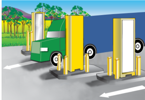
Figure 3.1: Illustration of a Radiation Portal Monitor. Image from [67].
