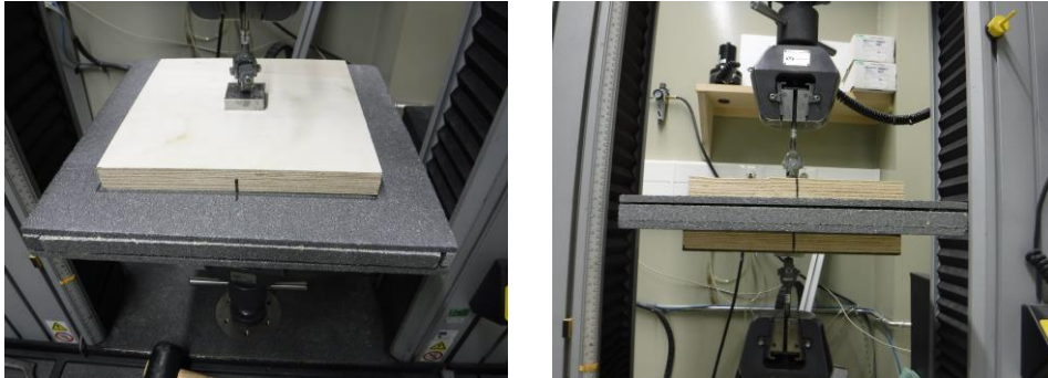
Figure B.22: Test specimens during tensile strength test.
