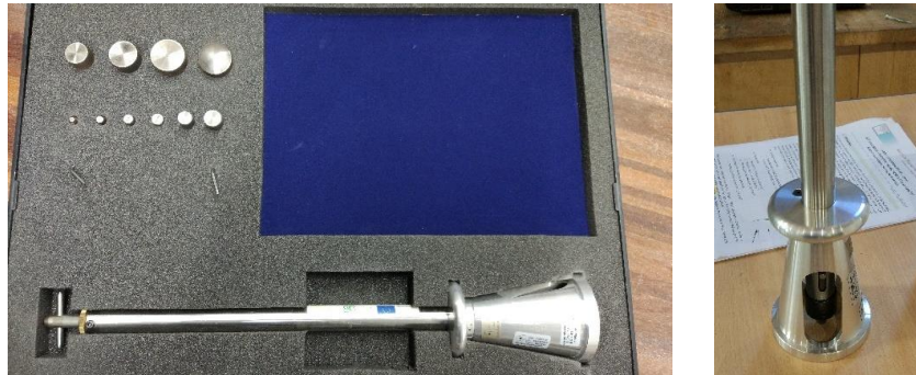
Figure B.7: Perfotest equipment with 10 indentors.
