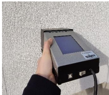
Figure 5.2: Determination of finishing coat emissivity by means of TIR100-2.
