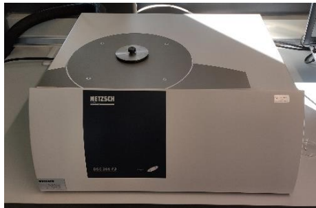
Figure 3.6: Differential scanning calorimetry apparatus for specific heat capacity determination.
