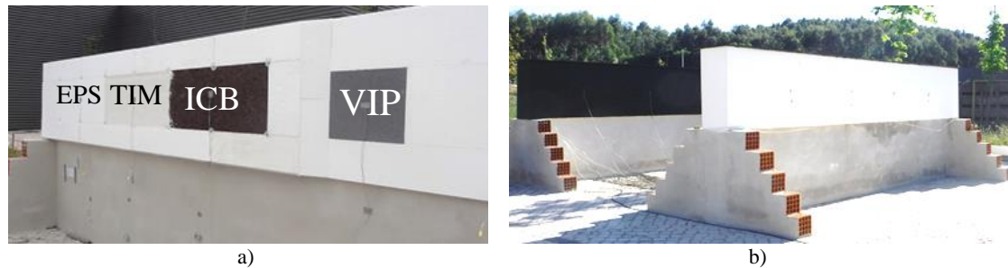
Figure 5.1: ETICS walls: a) different thermal insulation materials (EPS, TIM, ICB and VIP); b) different colour finishing coat (black and white).
