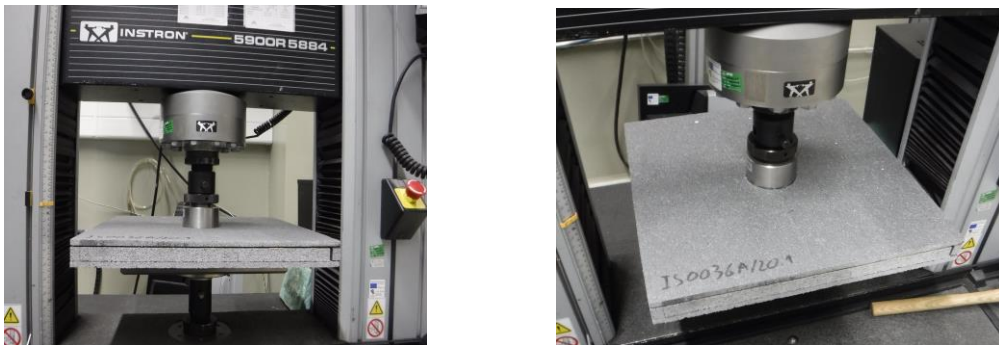
Figure B.15: Specimen 1 during point load test.
