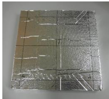
Figure B.10: Test specimen used for dimensional stability measurements.
