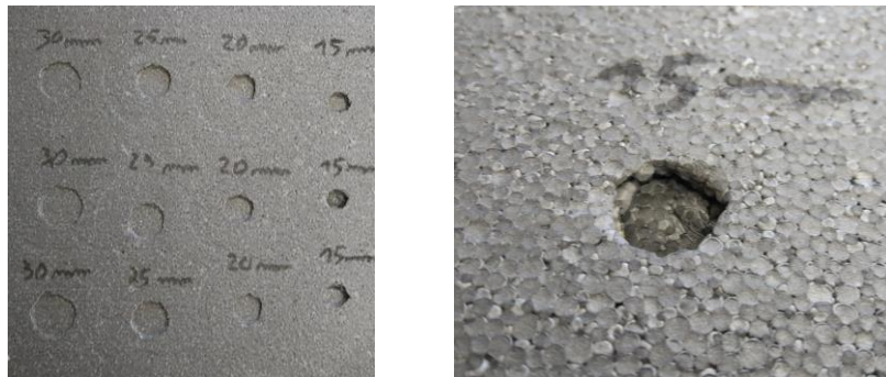
Figure B.20: VIP ETICS test specimen after perforation impacts.
