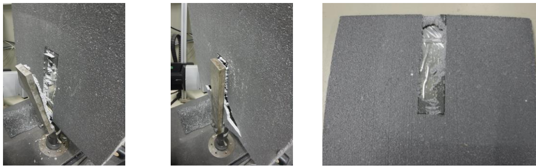
Figure B.19: Specimens after shear strength tests.
