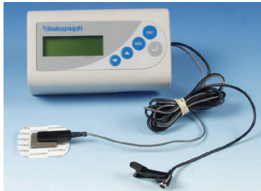
Figure 2.10: VitaloJAK cough monitoring device, with both lapel and contact microphone attached. From [Smith,2008].
