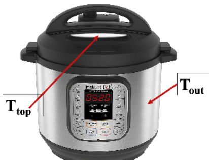
Instant pot pressure cooker (for shiro T in measured inside the cookware)
